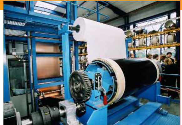
The process of coil-coating highly selective solar absorbers using the self-constructed sputtering plant at the Interpane factory in Lauenfoerde, Germany. (Source: Interpane Solarbeschichtungs GmbH)
