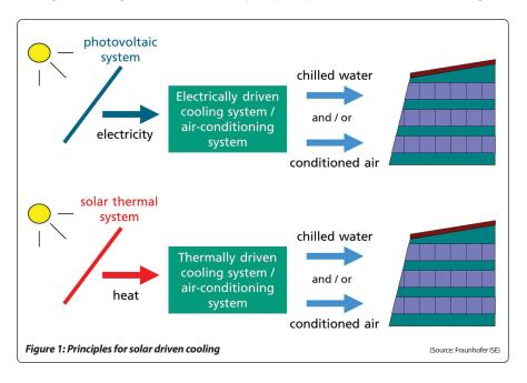
refrigeration systems using solar thermal energy as the main driving energy.
