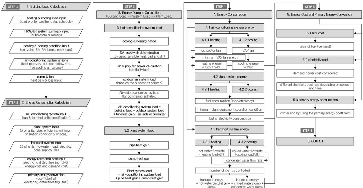
Fig. 7. A flow chart of the HVAC&R system energy calculation steps.
