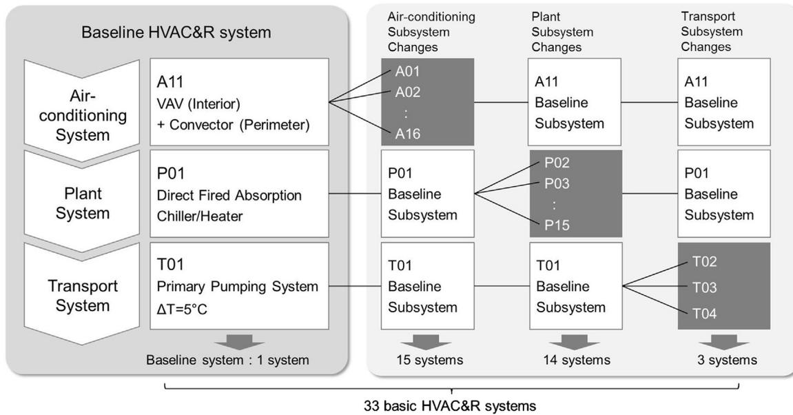
Fig. 6. A method for estimating the energy demand of basic HVAC&R systems.
