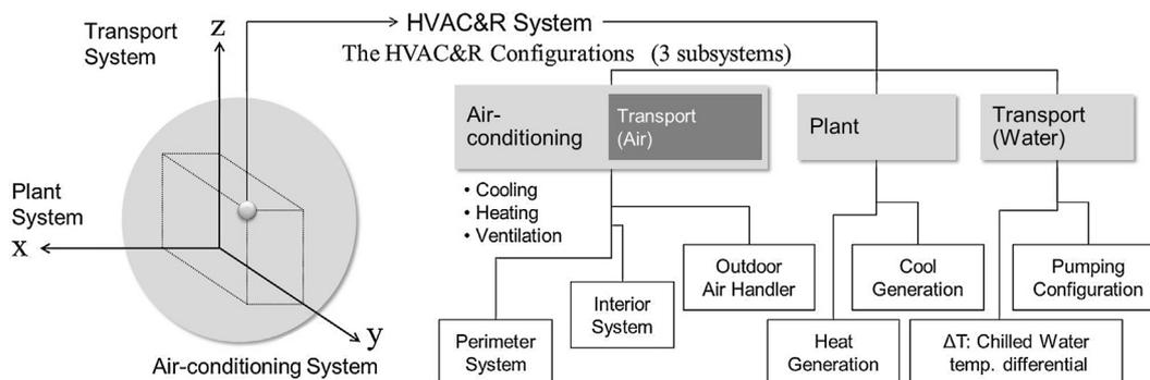
Fig. 4. The concept and composition of the HVAC&R system.
