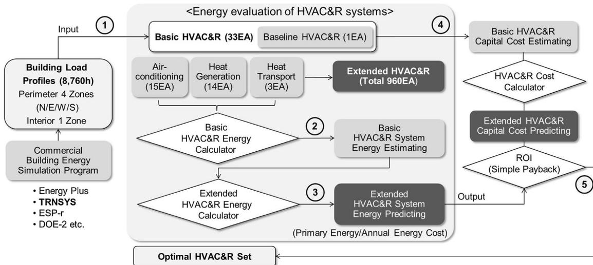
Fig. 10. A schematic flow chart of the major energy evaluation steps at the HEET.
