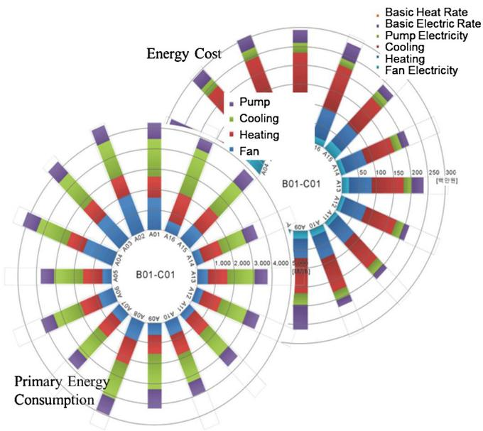
Fig. 16. An example of an energy performance map for HVAC&R systems.
