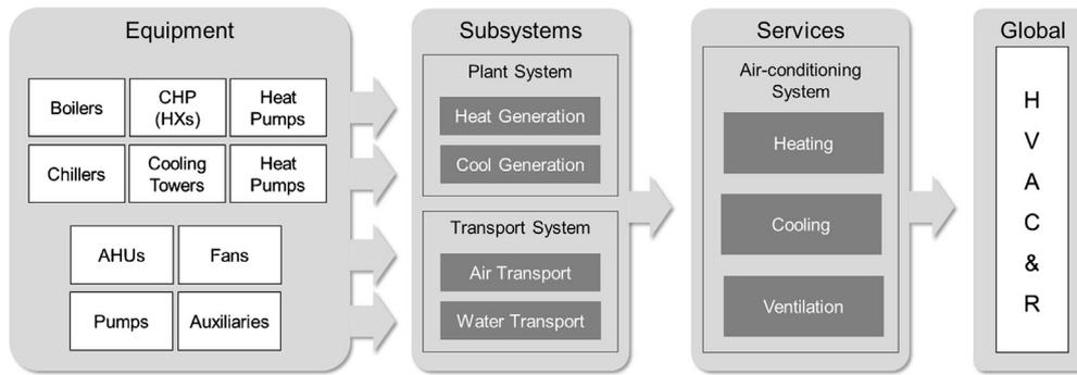
Fig. 2. HVAC&R systems energy use aggregation levels [9].
