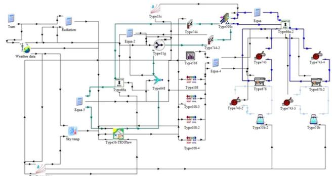
Fig. 13. TRNSYS model components and connections of set #1.
