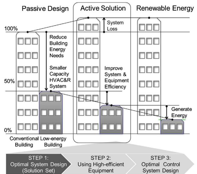
Fig. 1. Goal of building energy efficiency for HVAC&R system.
