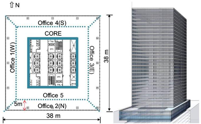
Fig. 12. An isometric model and typical plan of the case study.
