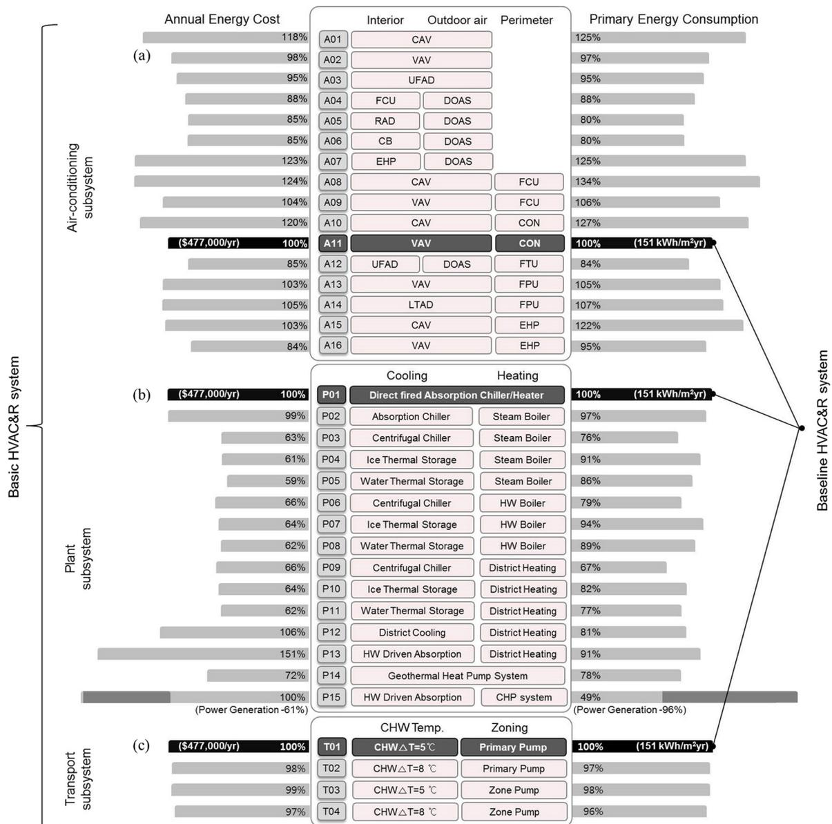
Fig. 14. Subsystem impact assessment for energy performance of HVAC&R systems; (a) air-conditioning systems, (b) plant systems and (c) transport systems.
