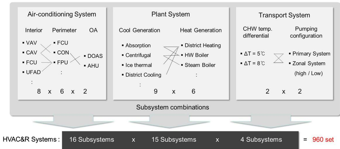
Fig. 5. Combination of all possible HVAC&R set configurations.
