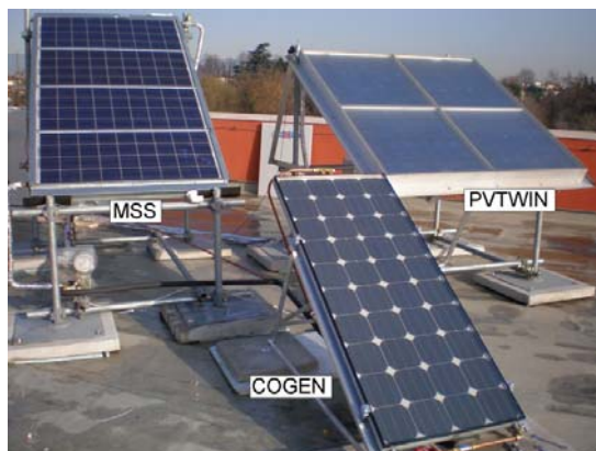
PV/T test stands at the University of Padova in Italy.
