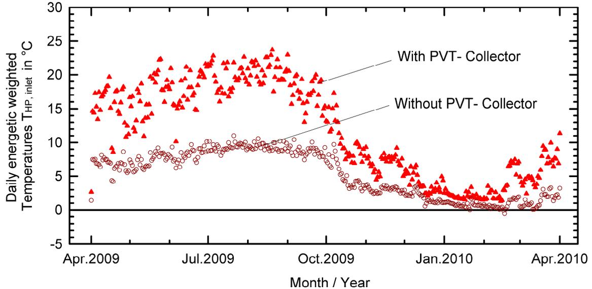
**Fig. 8: Daily average energetic weighted temperatures at the heat pump inlet  $T_{HP,inlet}$  for a pilot system (user heat demand 35 MWh/a, 12 kW heat pump, 39 m<sup>2</sup> PVT-Collector, 3x75 m coaxial BHE) in the first year of operation (with PVT-Collector: validated simulated data; without PVT-Collector: extrapolated data) (BERTRAM et al., 2011)**
