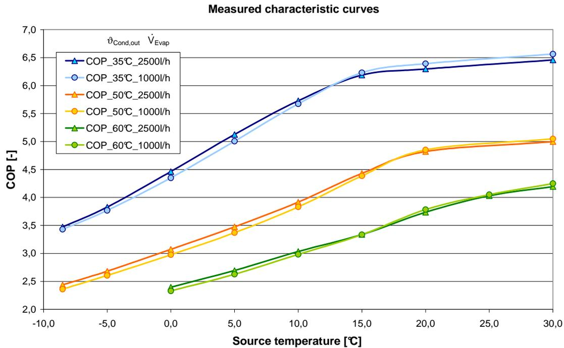
**Fig. 9: Measured characteristic curves of a heat pump at 3 different heat sink temperatures, each with 2 evaporator flow rates**
