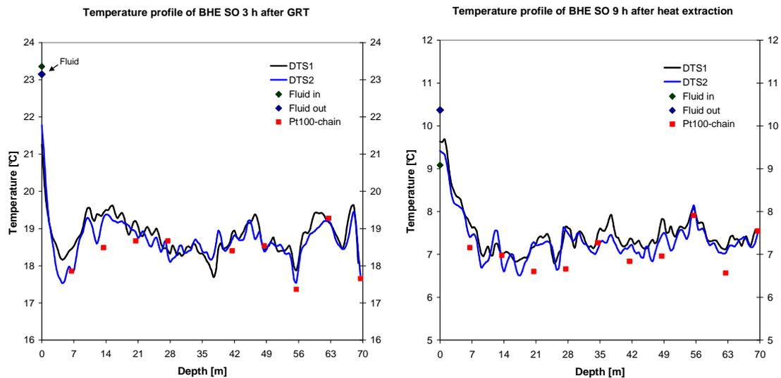
**Fig. 7: Comparison of DTS and Pt100 chain 3 h after GRT (left) and 9 h after heat extraction (right) on the BHE SO**
