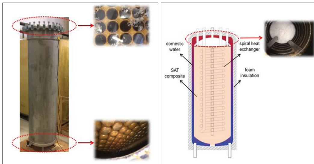
◀ **Figure 2. Cylindrical heat storage units:**
