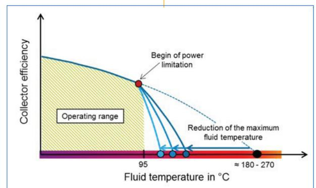
▲ Figure 3. Example of an efficiency curve of a solar collector with overheating prevention.
