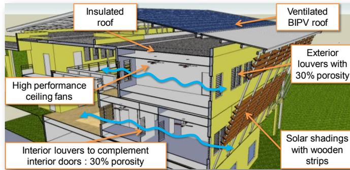
**Figure 1** Main features of the Enerpos building: passive design such as cross natural ventilation, solar shadings and insulated roof.
