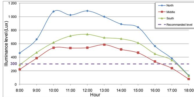
Figure 5 (a) Distribution of the three daylighting zones and location of the 12 desks on the classroom. (b) Graphic representing the average illuminance level for each zones during every hours from 8 am to 6 pm on a cloudy summer day.
