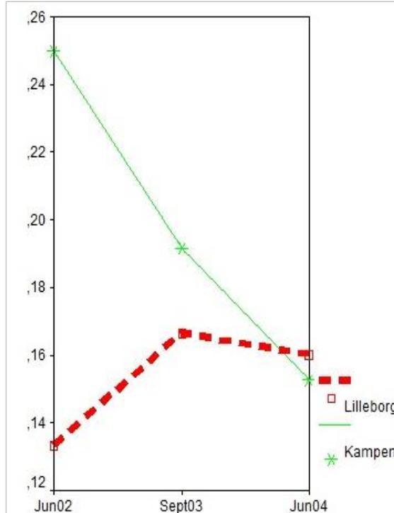
Figure: Result of a survey of Sick building syndrom-symptoms before and after renovation on Kampen School. The symptoms are reduced after renovation of Kampen. Also shown result of the reference school Lilleborg
