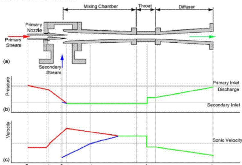
Figure 18 Typical ejector cross-section, pressure and velocity profiles along an ejector operating in critical mode. Primary, secondary and discharge streams are indicated in red, blue and green respectively. Adapted from Chunnamond & Aphornratana (2004) pump.
