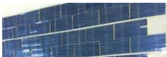
**Figure 12** A 0,1 m<sup>2</sup> flexible module capable of generating over 14 W.
