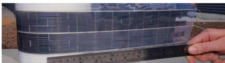
**Figure 14** Module can be flexed to radii of curvature smaller than 5 cm.
