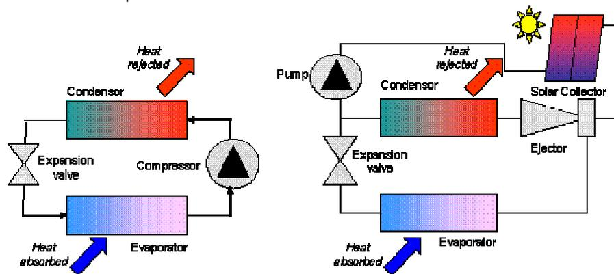
Figure 17 Solar driven ejector heat pump compared to a conventional electric heat pump.
