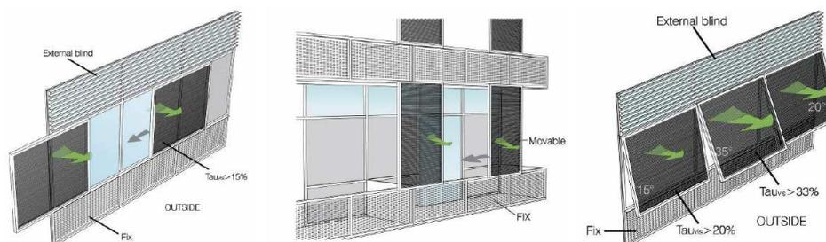
**Figure 10** The illustrations present three ideas for façade integration of the angle-selective glazing as external shading or as tilted windows.
