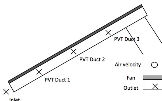
Figure 21 Schematic of thermocouple and air velocity sensor location
