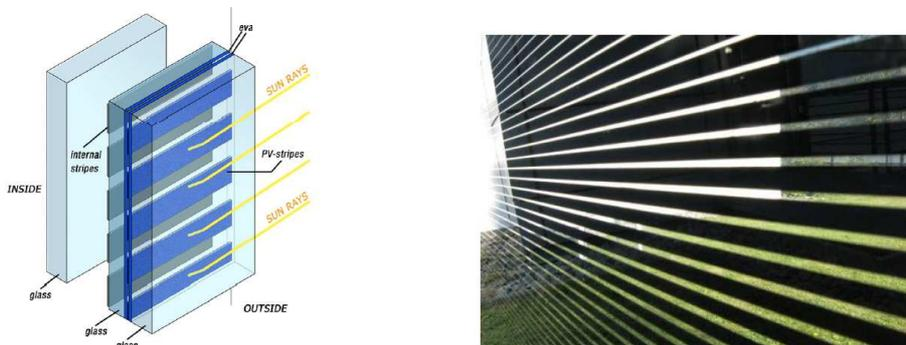
**Figure 9** Left: schematic view of the new transparent, angle-selective façade. The stripes (represented in blue) can be produced with photovoltaic technology. On the right: a detailed view of the first prototype with black ceramic frit stripes.
