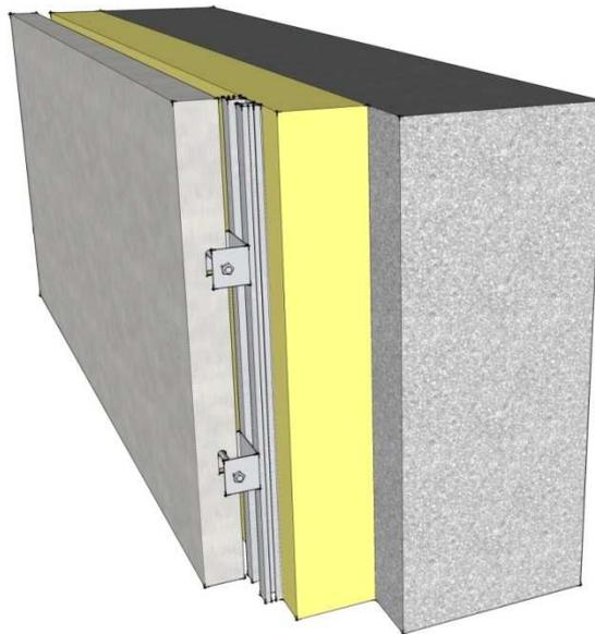
**Figure3** The rendering shows the preliminary sketch of the prototype of the innovative solar façade designed by EURAC in partnership with CGA, ARTAL ITALIANA, Frener&Reifer.
