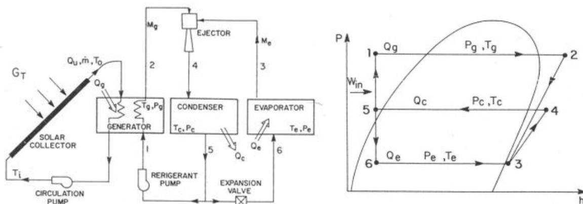
Figure 19 Solar powered ejector based solar cooling system (Sokolov, 1993).
